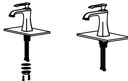
4. Reinstall the rubber washer, followed by the metal washer and lock nut. Hand tighten, then tighten further using a screw driver to tighten the lock nut.
