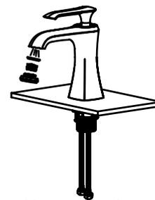
6. Remove the aerator and turn on the faucet for 1 minute to flush debris from faucet and feed lines. Turn faucet off and reassemble aerator.
