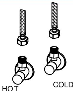
5. Attach flexible hose to the water supply.
