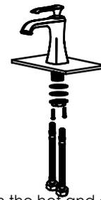
2. Screw and hand tighten the hot and cold flexible hoses to the faucet. DO NOT use a wrench to tighten hoses, as this may damage the hose and/or hose threads
